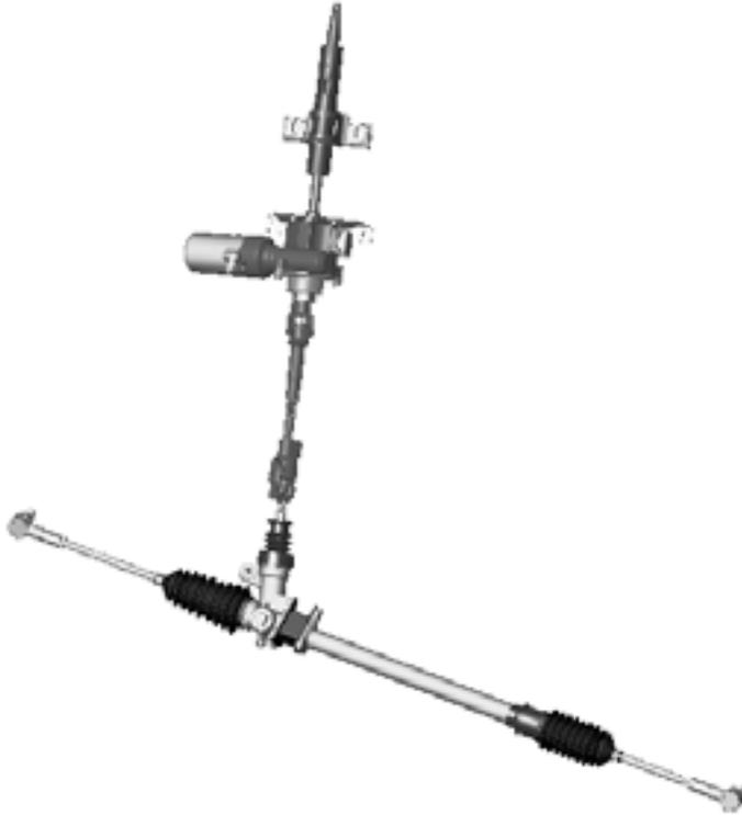
For many years power steering technologies were focused on hydraulic systems. However, demand is now shifting towards electronic power steering mainly due to logistical and fuel consumption benefits. The electronic power steering gear does not require a hydraulic pump, hoses, a hydraulic piston on the rack, or a sealed rack housing. It completely eliminates hydraulic fluid and the accompanying components of a hydraulic power steering gear.
