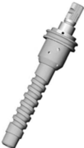
*Diagram 11: Rotary valve of a power rack-and-pinion steering gear*
